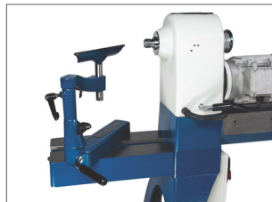
MACHINED HEADSTOCK END TO ATTACH 16" EXTENSION*
